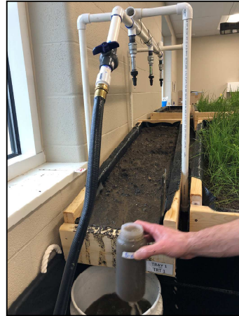
Figure 1. Runoff sample collection from replicate of “Bare Soil Dirt” treatment.
