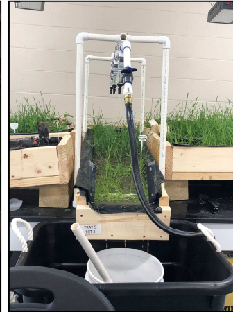
Figure 2. Rainfall simulation conducted on replicate of the “CSWS” treatment.
